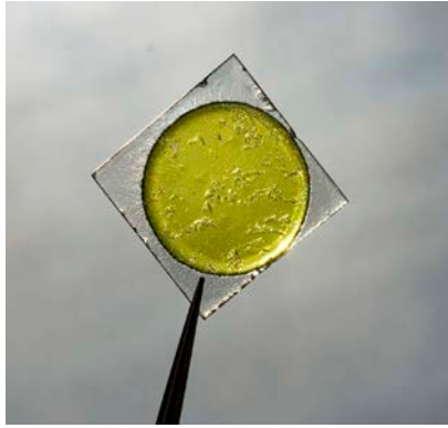
Figure 2. Cubic silicon carbide is a polytype that can further explore the graphene on silicon carbide properties.
